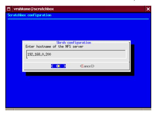
We need to specify the IP-address that is assigned to the Scratchbox host in the USB network. In this example it is the gateway: 192.168.0.200.
