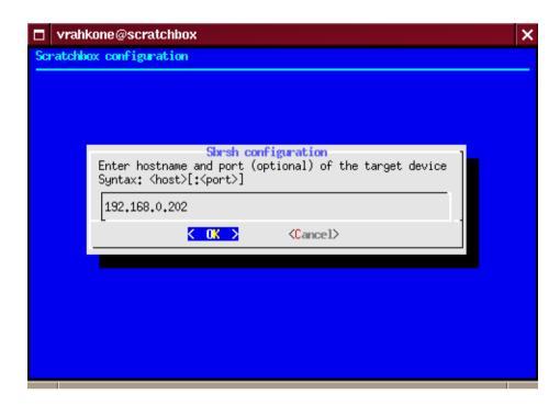
In our example the device has been connected to the Scratchbox host via a local USB network and we have assigned the IP-address 192.168.0.202 for it. We are running sbrshd at the default port (1202) so we don't need to specify it.
